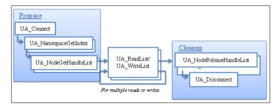
However, because each unique MDIS valve object has unique identifiers for each of its information model components, a custom configuration is required for each valve. That is, the OPC identifier for say, the "Fault" component is different for every valve, and function block configuration in the workflow depiction above needs to be adjusted for each valve accordingly in order to read the value of "Fault".
