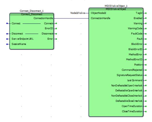
The MDISValveObject custom function block shown was developed using the 61131-3 structured text programming language. Internally the block uses these PLCopen function blocks<sup>4</sup>:
